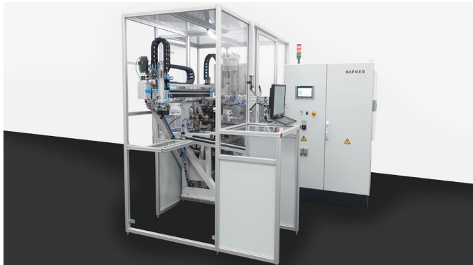
The measuring device for differential cases conducts tactile determinations of diameter, length, form and position tolerances, as well as axial run-outs. Both static and dynamic.
