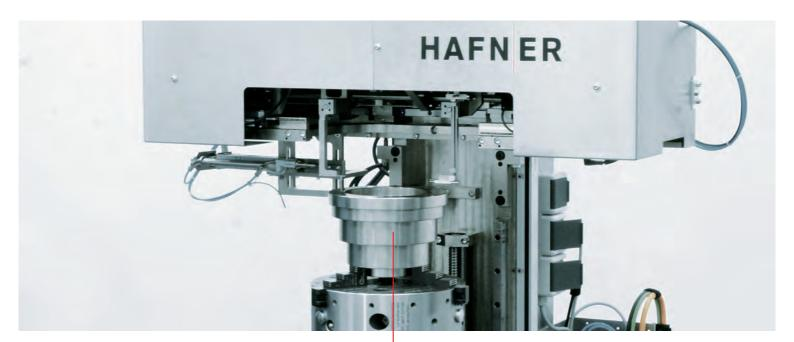
The GEAR CONTROL is on a base frame with vertical workpiece arrangement. The sequence control can be run via the control of the machine tool or an independent controller. Equally, the evaluation of the measuring sensors can be either with machine tool's control or an additional measuring computer.
