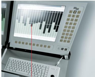
The measuring computer evaluates the measurement data and displays the results. Besides this it also controls all movements within the POLARIS. Influences due to changing workpiece and/or ambient temperatures will be equalled with temperature compensation.
