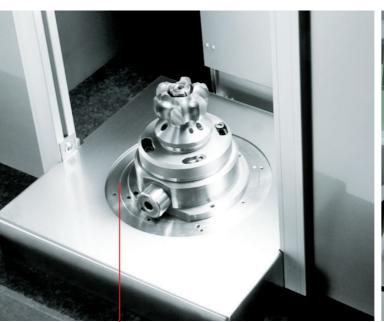
High-precision, air-supported rotary table with torque drive and internal wobble error < 0.1  $\mu$ m. Built on a massive vibration damper decoupled granite plate. A workpiece holder is mounted on the rotary table ensuring a stable component fixation during the entire measurement.
