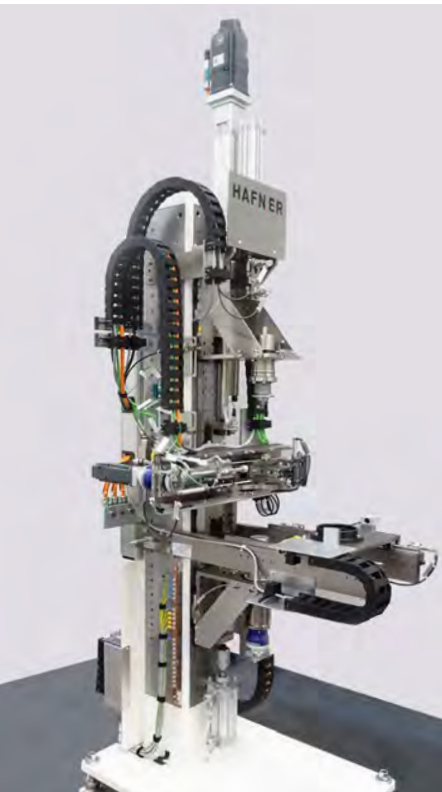
Vertical ShaftControl offers high flexibility for precisely checking all rotationally symmetrical workpieces. It is available in different versions, and can be optimally adjusted to custom requirements.
