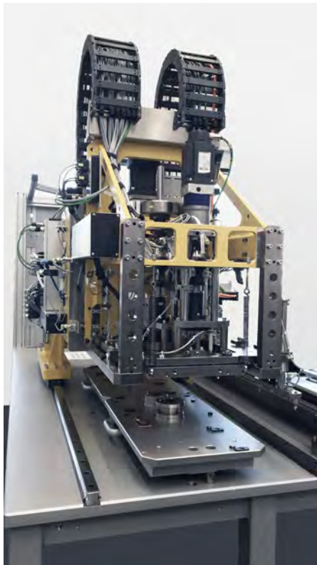
The solution for E-gears measures adjusting washers and sealing profiles, as well as the thickness of washers and sealing profiles on gears and housings, including adjusting washer magazine.
