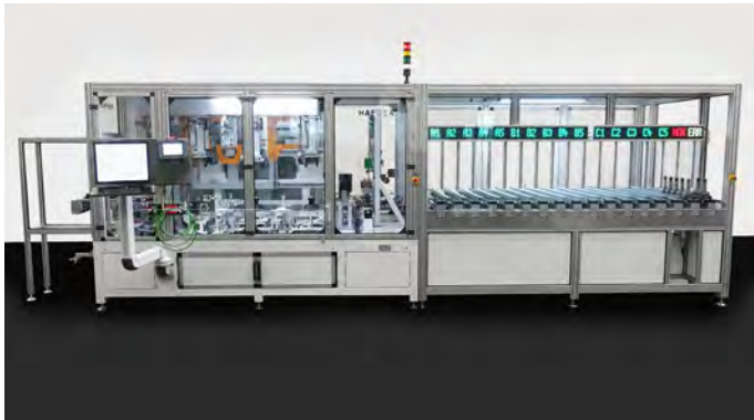
The measuring device for kingpins conducts tactile and static diameter measurements (double sphere dimension, pitch circle, gearing) and angle divisions.
