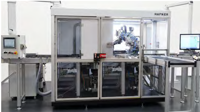
The measurement and testing machine for truck brake discs allows for 100% controlling, detects even the smallest errors, and precisely measures diameters, lengths and dimensional tolerances.
